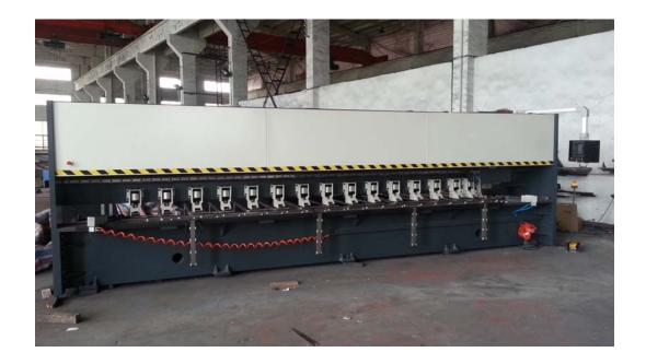
the GBC V grooving machine GBC-1250x4000 is a kind of latest development equipment, it adopt the steel wire as its transmission system. It instead of the gear, rack and pinion and ball screw, to realize flexible drive. It completely avoid the vibration cased by the rigid connection of rack and pinion. And significantly improve the roughness of groove surface and product quality as well.
