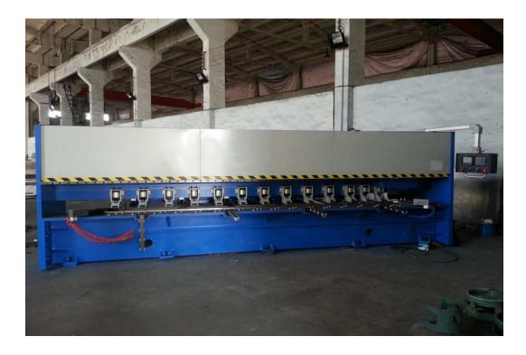
The SBC V grooving machine is used to make a slotting on the sheet metal to get the sharp edge angle after bending , the machine adopt precision ball screw and linear guide way as its transmission, and has high machining accuracy, so it is particularly significant for high class-products. This structure is universally used on relevant equipment in foreign countries.
