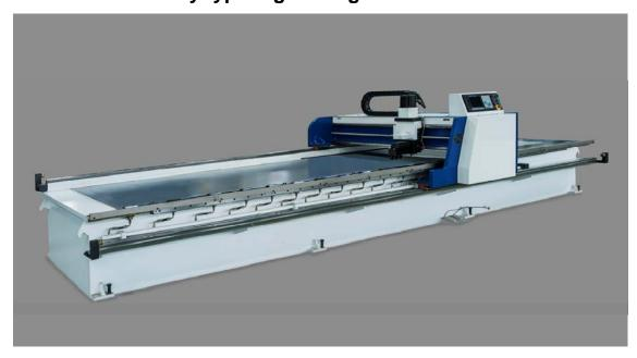
LBC gantry type V grooving machine LBC-1250X4000 is improved from the conventional table type grooving machine. The V grooving machine has all the advantages of conventional table type grooving machine( such as the sheet is fixed& static. No scratches on its opposite during grooving, simple structure and good rigidity and better stability).
