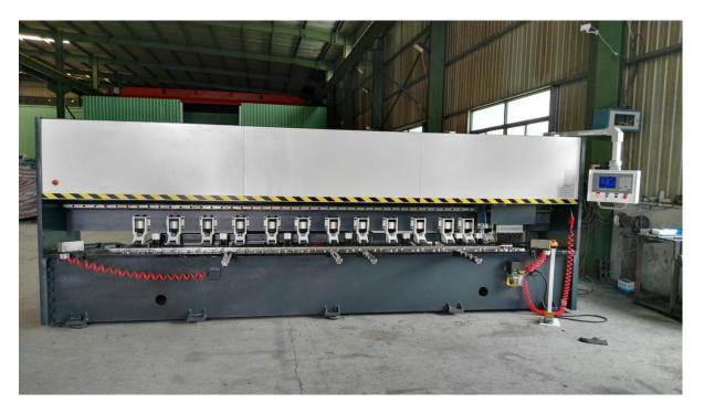
the GBC V grooving machine GBC-1220x4000 is a kind of latest development equipment, it adopt the steel wire as its transmission system. It instead of the gear, rack and pinion and ball screw, to realize flexible drive. It completely avoid the vibration cased by the rigid connection of rack and pinion. And significantly improve the roughness of groove surface and product quality as well.
